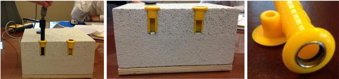
1. When installing testing sleeves, you must first drill to the proper depth.
