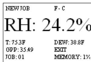
2. **The meter will begin taking readings.** As a default setting the RH reading will be the most prominent on the screen. If you would like to make another variable (temperature, GPP or dew point), the prominent reading, use the ↑ ↓ and ⇐ ⇒ keys to highlight your selection. Press the **SELECT** key to choose that variable.
