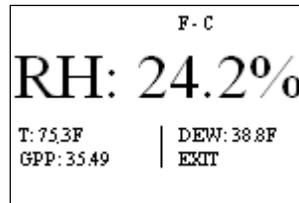
2. **The meter will begin taking readings.** As a default setting the RH reading will be the most prominent on the screen. If you would like to make another variable (temperature, GPP or dew point), the prominent reading, use the  $\uparrow$   $\downarrow$  and  $\leftarrow$   $\rightarrow$  keys to highlight your selection. Press the **SELECT** key to choose that variable.
