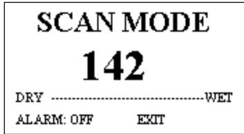
2. **You may begin taking readings** by firmly pressing the back of the meter onto the material. This will display a relative reading that ranges between 0 and 300.
