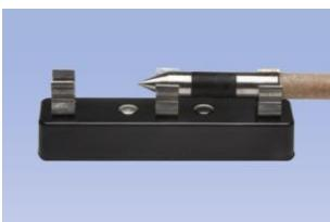
**MCS-4** - This moisture content standard is great for verifying that your F-series moisture meter is in calibration. With two electrical resistance values (16% and 22%) to test your meter against, you can be sure that your readings will stand up to the strictest standards of accuracy.
