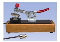
Other electrodes, such as the 43-E clamp electrode, can be used for checking moisture in finished paper products or thin sheet stock.
