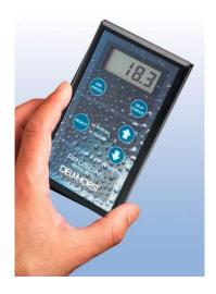
With built-in species corrections, it is possible to program the meter to adjust its readings based on the SG of the wood being tested. This makes ProScan ideal for flooring installers, flooring manufacturers, furniture manufacturers, and any other professional who has to work with a large variety of wood species on a daily basis.
