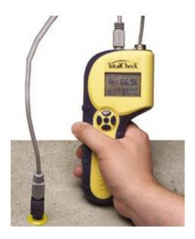
With all of these problems susceptible to a wet environment involving concrete, it's advised that you use a concrete moisture meter on your next project. Some suggestions include the **TotalCheck 3-In-1** moisture meter or the **HT-4000F** stand-alone thermohygrometer, which both comply with the ASTM F2170-11 standard.
