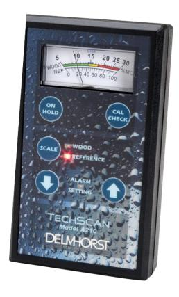
One of the best ways to use a reference scale meter is to take a reading from an unaffected sample of material that is known to be dry first. Once you have a reading from the "dry" sample, use that reading as the baseline for the readings you get for that material for the rest of the job.
