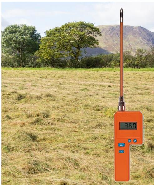
For example, when testing the **moisture content of hay**, hay growers can use a test method called the oven dry test, where a sample of hay is weighed, placed in an oven to be dried out over the course of several hours, and then weighed again, a process that repeats until the hay no longer changes weight. The problem here is that, while highly accurate, this process takes hours, which is time that could be dedicated to other tasks.
