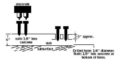
If the meter still indicates green or "dry" the floor is ready for covering. Tests should be made at several points, especially when the slab is thick and air circulation is poor.
