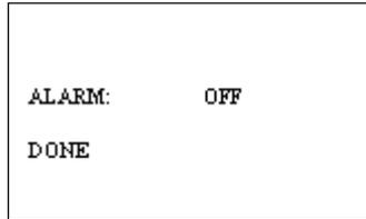
2. **The default status of the alarm is “OFF.”** Press the **SELECT** key to turn it on.
