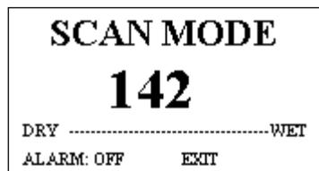
2. **You may begin taking readings** by firmly pressing the back of the meter onto the material. This will display a relative reading that ranges between 0 and 300. If you wish to hold a reading on screen, press the **SELECT** key; otherwise move the meter to another area to take continued readings.
