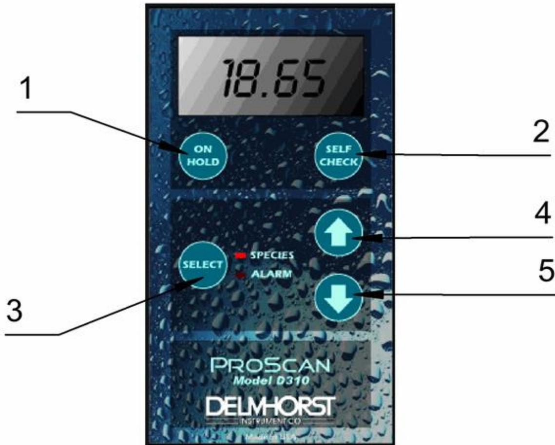
1. **On/Hold Key:** Press to turn meter on, return to reading mode after checking calibration, setting alarm, or to hold the current reading if pressed while reading. (There is a slow beeping sound while holding a reading.)
