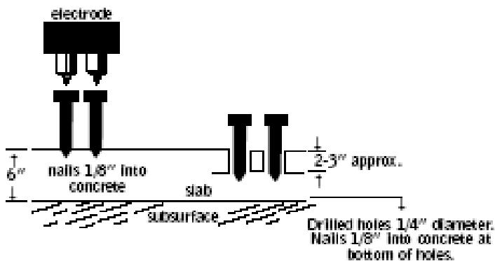
If the meter still indicates green or "dry" the floor is ready for covering. Tests should be made at several points, especially when the slab is thick and air circulation is poor. Tests should only be made in newly drilled holes, since the inside surface of the holes can dry out while the rest of the slab is still wet.
