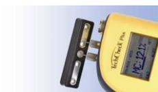
**MCS-1** - Moisture content standards are great for verifying that your Delmhorst moisture meter is in calibration. The MCS-1 can be used on any meter with a wood scale. With two electrical resistance values (12% and 22%) to test your meter against, you can be sure that your readings will stand up to the strictest standards of accuracy.
